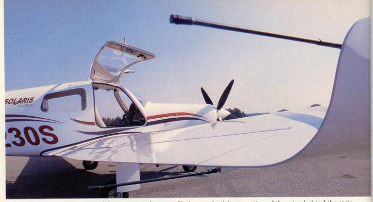
the windshield that forms part of the airplane's lightning protection system—in addition to providing rollover protection and support for the doorframes. While some carbon fiber is used around the doorframes for strength, the vinylester resin was chosen for the primary
